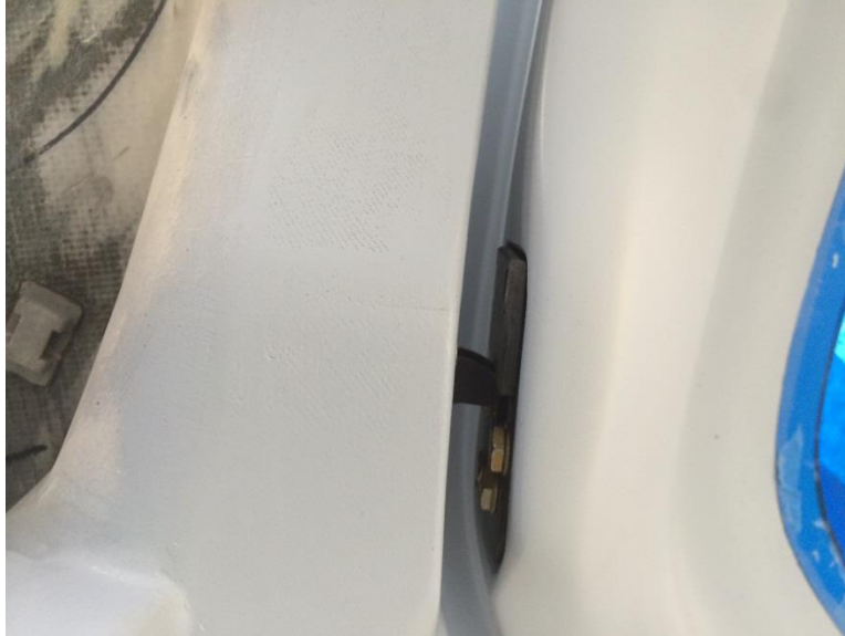
Photo Showing Claws and Striker Plate with Canopy Propped Open by Latch Mod
