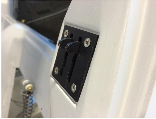
Photo of Canopy Latch Claws Modified to Remain Partially Extended When In Full Canopy Release Position
