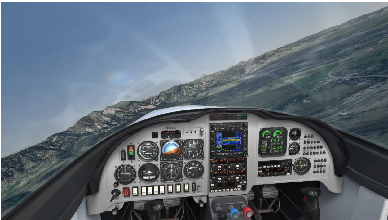
Legacy cockpit sight picture, visual pitch attitude reference
